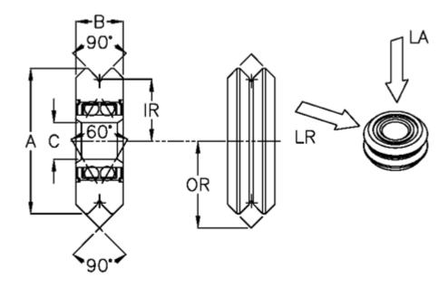
$\begin{array}{ll} \mbox{Diameter A} & = 30.73 \\ \mbox{Hole size C} & = 9.53 \\ \mbox{Internal radius IR} & = 12.70 \\ \mbox{Outer radius OR} & = 18.26 \\ \mbox{Width B} & = 11.13 \\ \end{array}$
